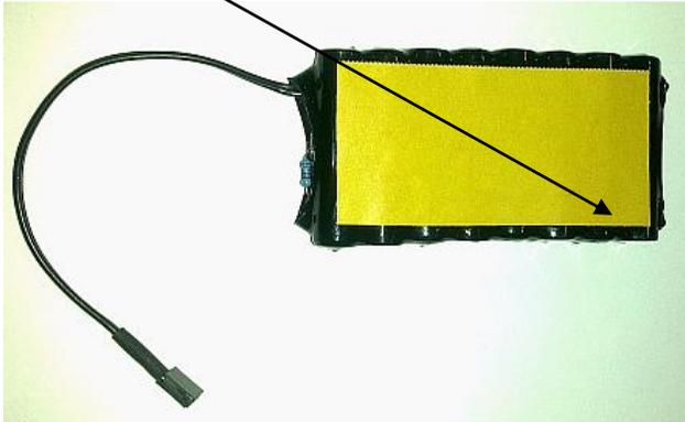
3. Fix the ACU pack into Gateway cabinet. CAUTION for holes for signalling LEDs! DO NOT COVER!
