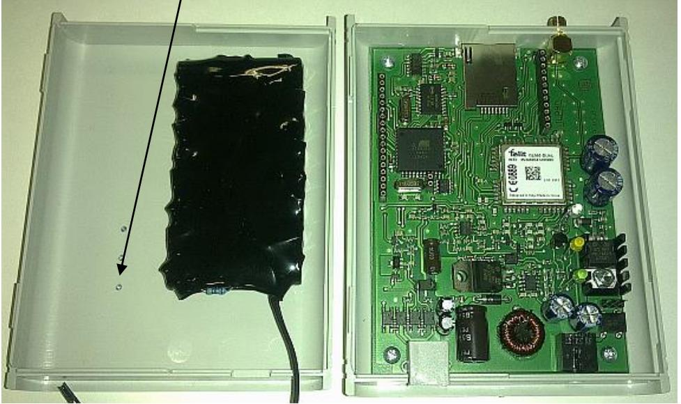
4. Rechargeable batteries may not be delivered in a charged state. Start the gateway first and wait for network log in. Then connect cable from ACU pack to appropriate connector..
