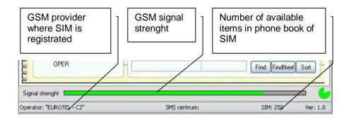
Program monitors communication microprocessor with GSM module. It shares this communication way to module. Microprocessor works with GSM module in 30 sec. period. It means that program has periodically 30 sec. For its own communication (loading or saving numbers) as same as SMS to SIM of the unit. This time is shown by green point in right this time program. Out down corner of of microprocessor works with GSM module) are some features unavailable.
