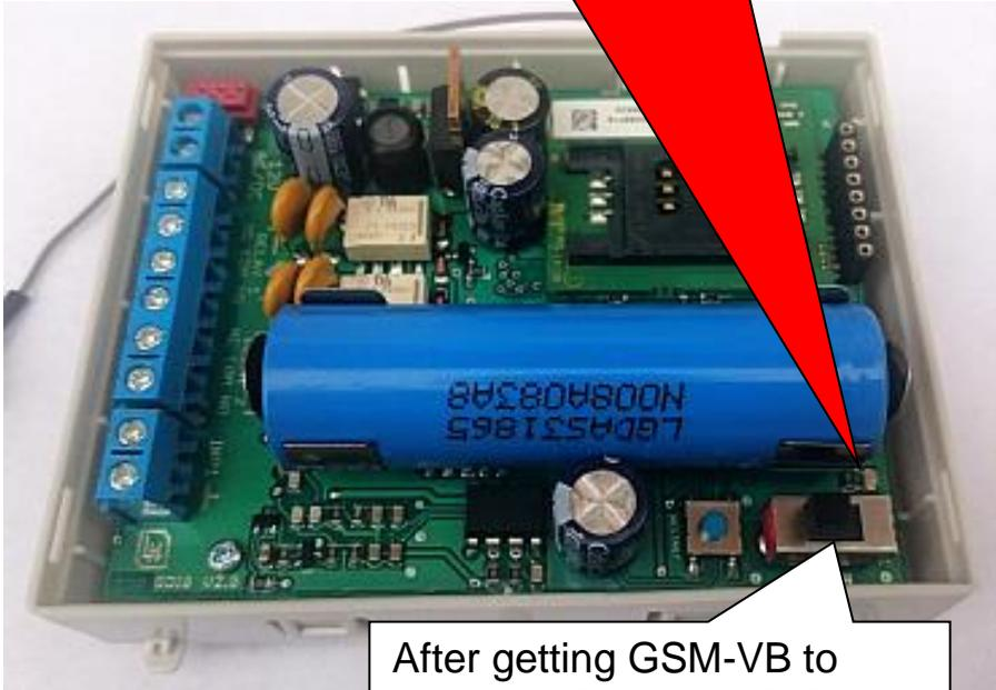
After getting GSM-VB to operation by turn switch to position ON you connect backup battery
