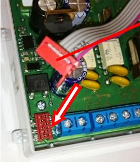
**K2 cable (cable with red connector)**
