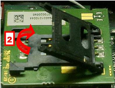
Insert the SIM in correct position (3) to the holder. Close the SIM holder (4).
