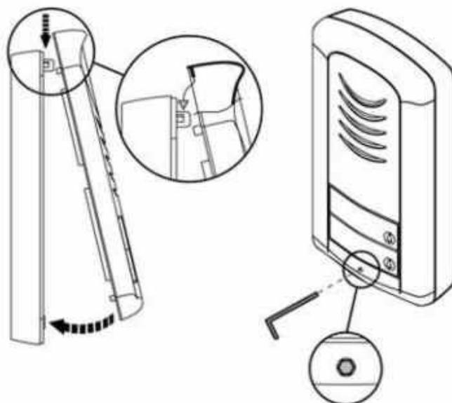
**CAUTION!** During assembly of front panel you might connect/disconnect speaker connector (via schematics)
