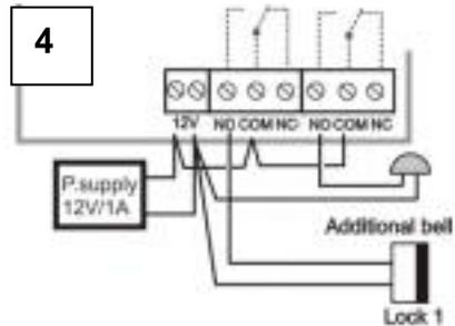
**CAUTION!** Relay contacts cant close 230V directly.To control directly 230V devices you must use contactor.
