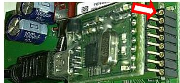
2. Remove front cover of GDI and insert connector of programming modul into GDI (via picture). On programming modul must light on red LED (It is flashing same way like yellow LED on GDI)
